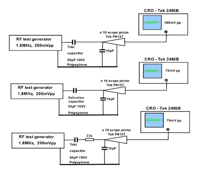
The tests, as shown above, indicated that the capacitor had gone high ESR to the tune of about 22k. Of course ESR meters cannot measure low value capacitors like this. Then I tried placing resistors of this value, in series with good low value capacitors in the range of 50 to 100pF, my YF-150 capacitance meter is unable to detect significant series resistance.
