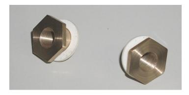
I bought some "plastic" replica knobs on ebay, but was disappointed with the quality. After a while I found some original metal knobs from another model of Astor transportable car radio. Almost perfect but the centre knob was designed to push onto a 1⁄4" shaft. This radio had 3/16" shafts for the centre knob, so I machined some brass inserts to fit into the centre knobs to make them compatible, these inserts are visible in the photo below:
