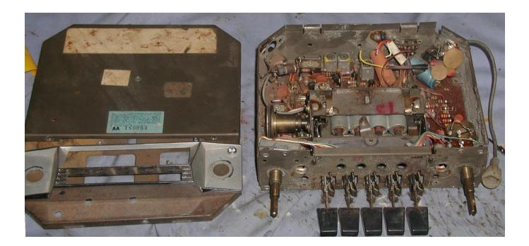
The radio was disassembled, this required removal of a number of rivets (replaced with identical ones later) to be able to disassemble the audio amplifier assembly heat sink assembly from the top metal lid.
