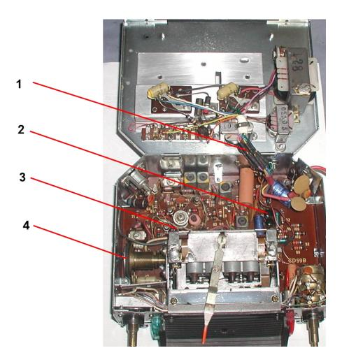
1) The upper panel (radios top lid) holds the audio amplifier assembly and it was linked by a leash of wires to the radio main board. For ease of restoration the wires were cut and 0.9mm gold plated pins and sockets were inserted (these are available from Jaycar) to make it easy to separate the audio amplifier and top plate assembly.
