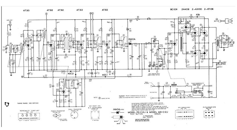
The transistors were drawn in a way typical of some early 1960's vintage radios. One interesting thing is that the audio driver transformer does not have a primary winding.
